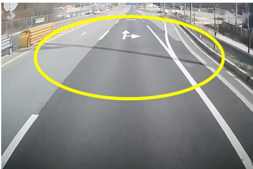
<Figure 1> Dump truck stopped because it recognized the shadow as an obstacle
