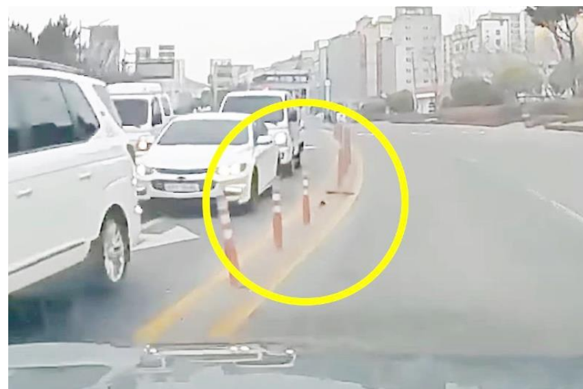
<Figure 2> Blocking stick recognized by FCA as human as an obstacle
